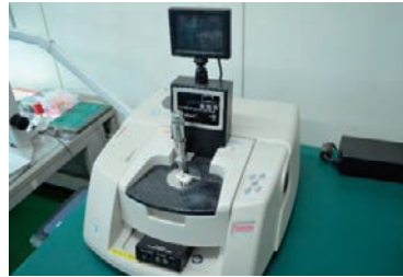
FT-IR (フーリエ変換赤外分光光度計) Fourier Transform Infrared Spectroscopy
