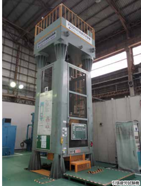
引張疲労試験機 Tensile strength fatigue testing machine for PC strand
