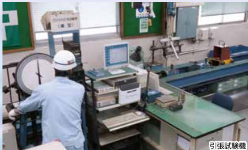
引張試験機 Tensile strength testing machine for PC strand
